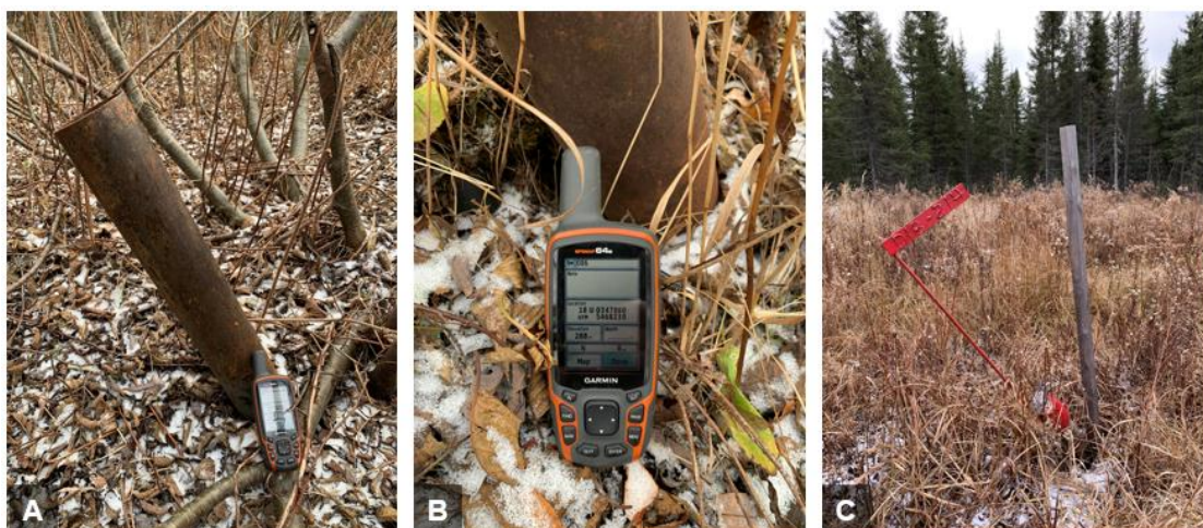
A) Casing left in place for drill hole D-11-209 from North American Palladium's 2011 drilling program; B) Casing left in place for historical drill hole BD-04-78 from Strateco's 2004 drilling program; C) Well identified collar with metal rod and flag for drill hole D-18-214 from the issuer's 2018 drilling program. (QP site visit, November 8, 2022).
