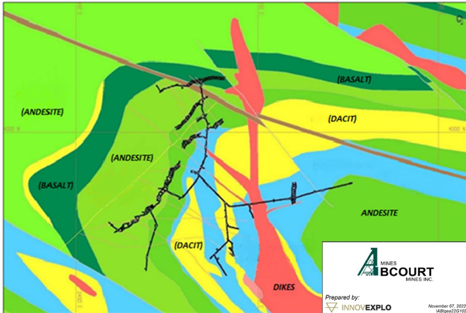
Figure 7-5 Plan view of level 665 showing development (note the angular relationship of the development with respect to geological contacts)
