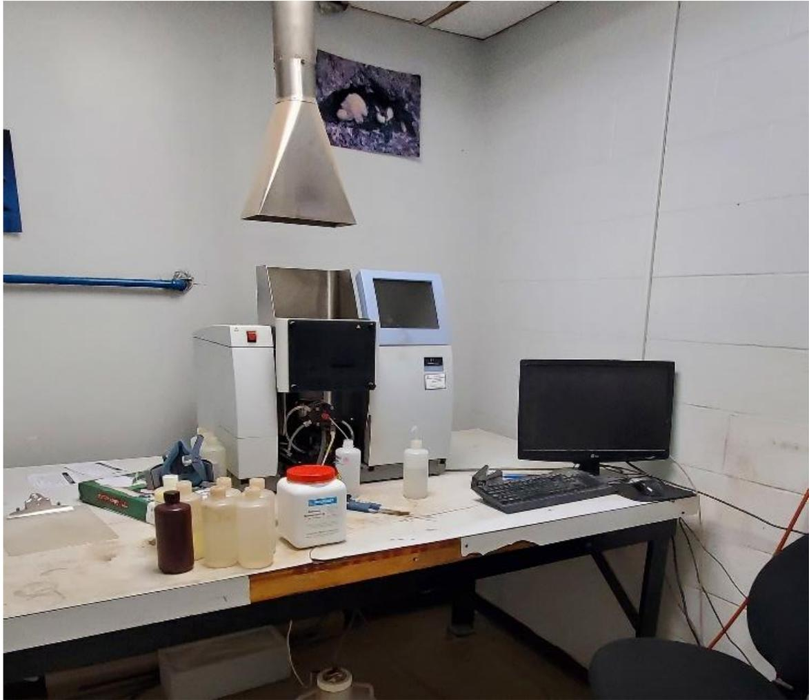
**Figure 12-3 Atomic absorption instruments**
