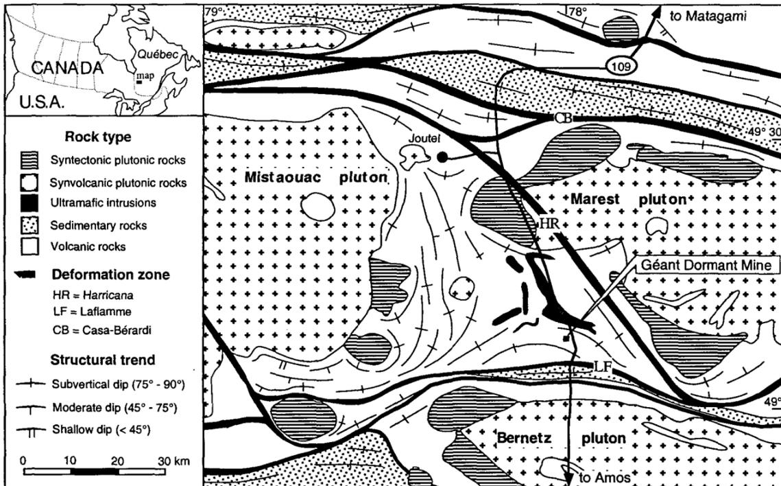
**Figure 7-1 Simplified geological map of the mine district showing the location of the Sleeping Giant gold deposit close to the central part of a triple junction of structural trends. Map modified from Hocq (1990) and Chown et al. (1992).**
