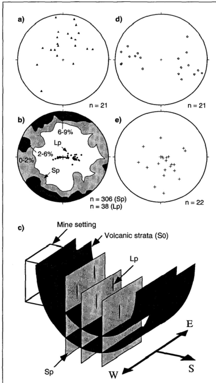
(a) Equal area projections (lower hemisphere) of Sp planar fabric and Lp stretching lineation. (b) Schematic structural setting of the deposit
