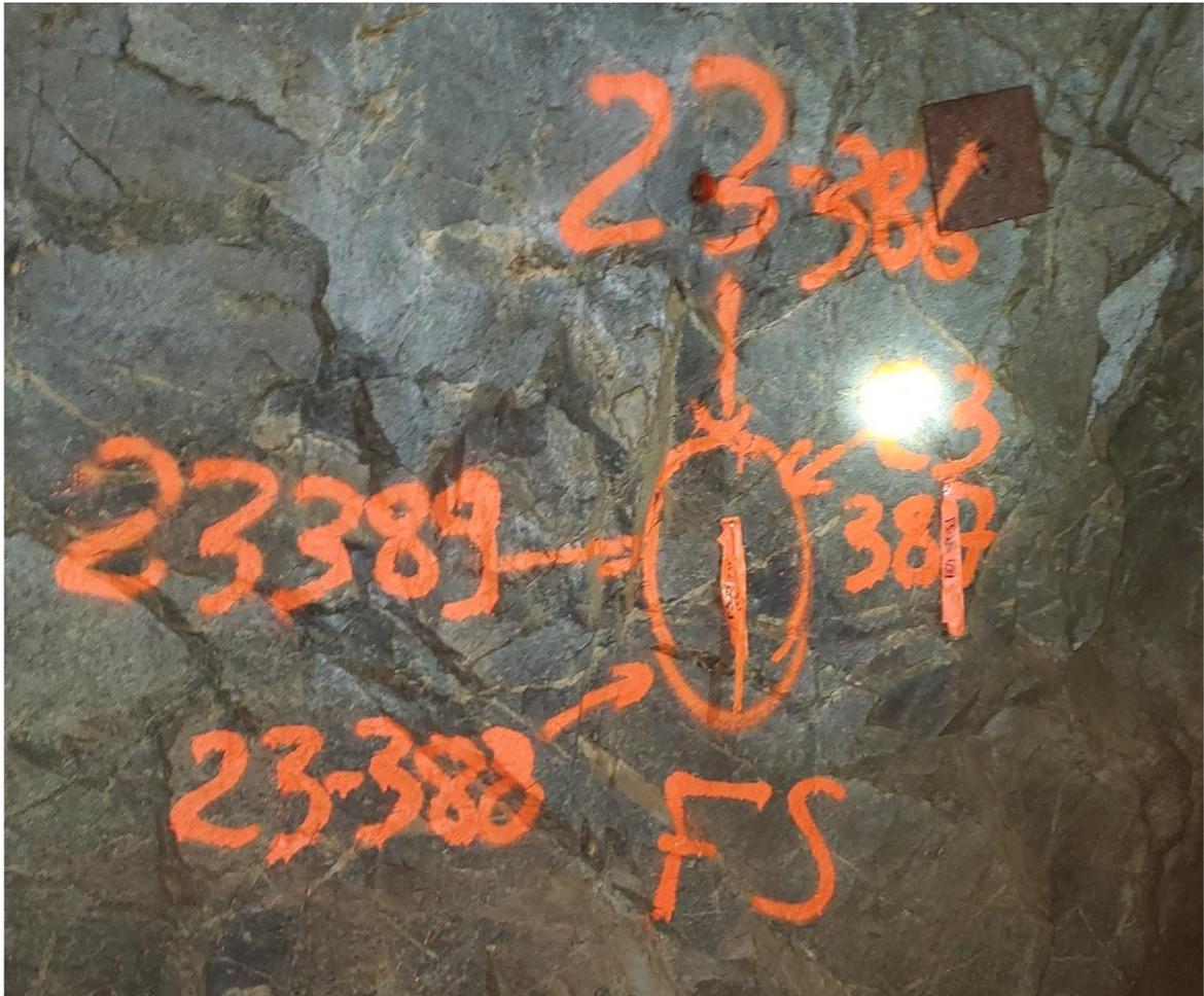
Figure 10-3 Front-sight for underground drill hole collar surveying
