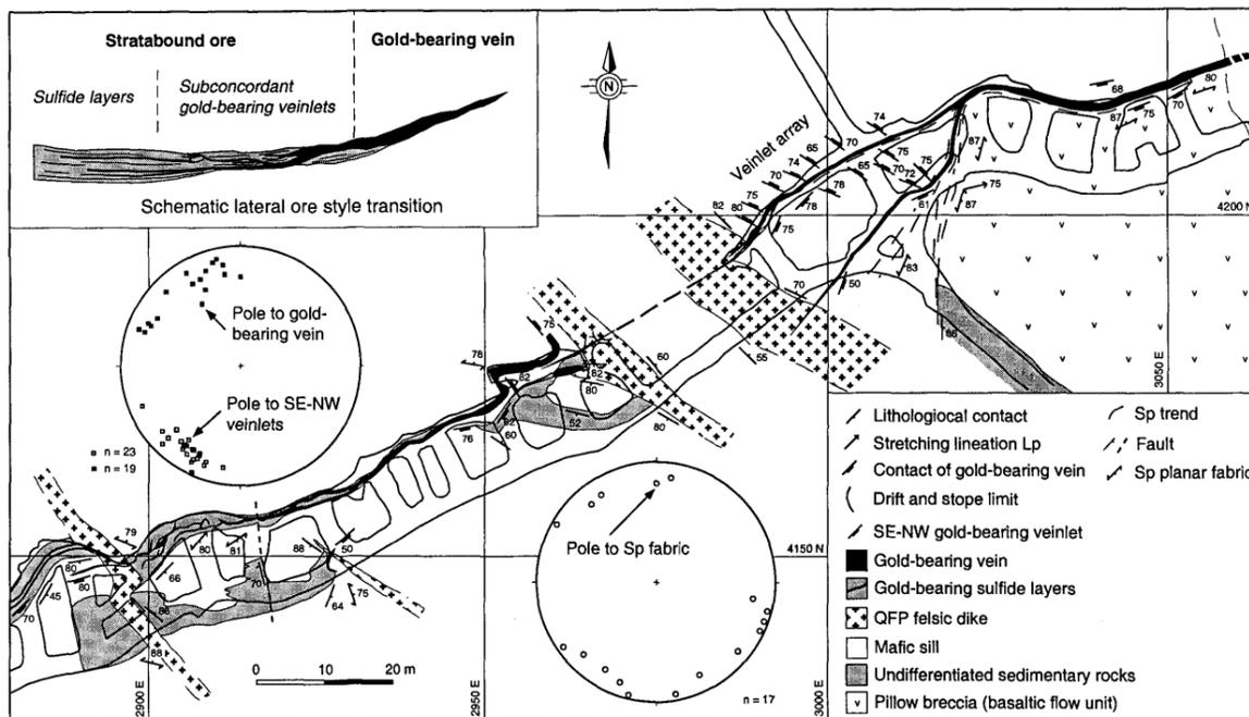
**Figure 7-11 Detailed geological map of the entire 20E-20W zone at level 355.**
